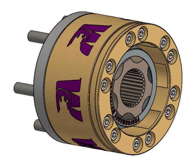
NOTE: THESE CV JOINTS ARE LARGER IN DIAMETER THAN A 930 CV JOINT AND WILL NOT FIT INSIDE FLOATING STYLE HUBS
